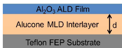
Figure 8. Schematic of alucone interlayer with variable thickness between an \text{Al}_2\text{O}_3 ALD film and a Teflon FEP substrate.
